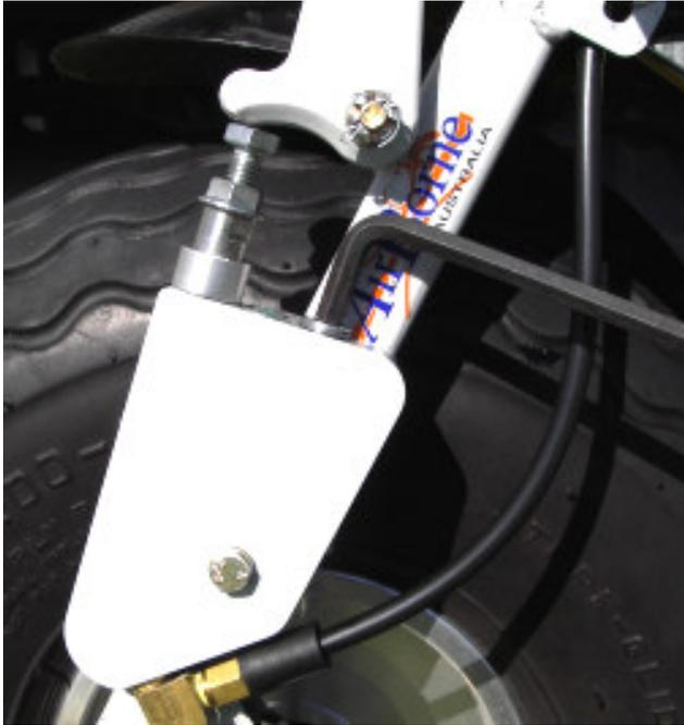
Figure 1 Brake master cylinder, remove reservoir plug
