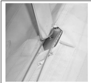
Remove king post base padding and plug the kingpost into the socket on the rear most hole of the keel. Make sure that the cross bar wires are not twisted and are on either side of the king post.
