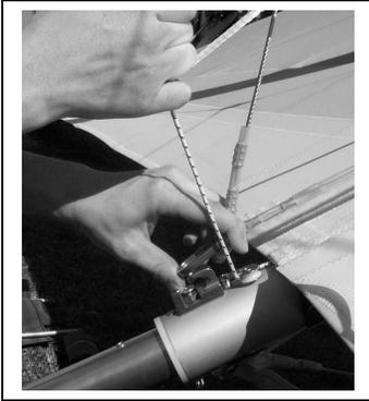
Depress quick clip with left thumb. Use right hand to pull on the webbing handle. Remove the shackle from the quick clip block and allow webbing handle to move forward.
