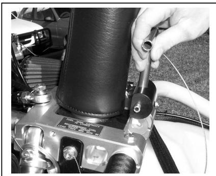
Insert the lever so that the flat section is facing toward the mast.
