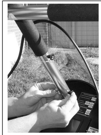
Figure 20 Section 4. Insert Mast Lever
