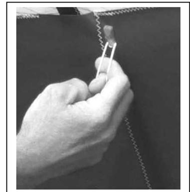
Figure 11 Section 4. Insert Remaining Sail Battens
