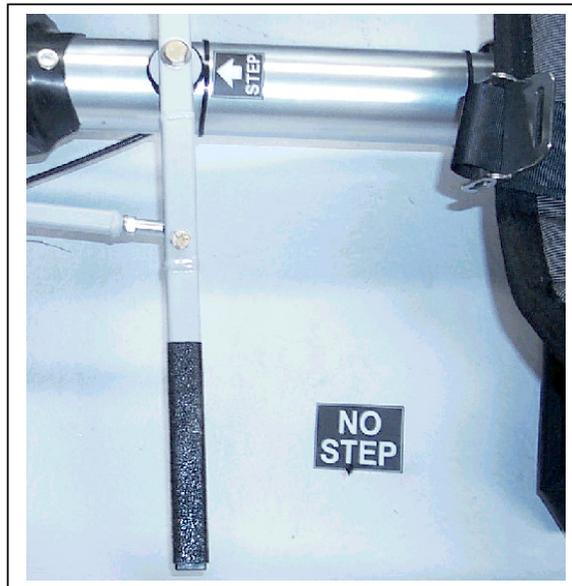
Figure 5 Section 2. Step and No Step Placards
