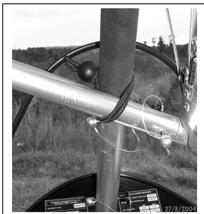
The aircraft should be parked in a crosswind position with the wings base tube secured to the mast brace with the bungee supplied.
