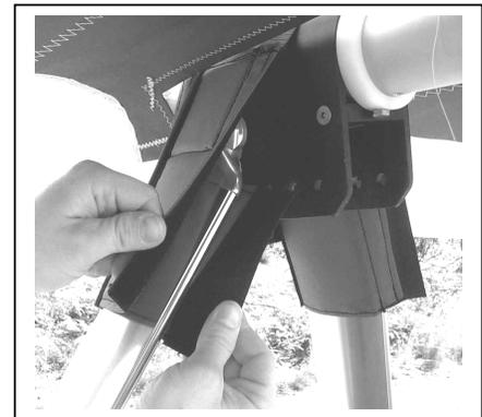
Figure 28 Section 4. Fit U-Bracket Cover
