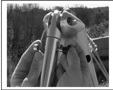
Remove control bar and down tube padding. Spread the control bar down tubes out and insert the base bar onto the alloy knuckle. The pip pin is then inserted from front to back. Ensure that the pip pin end cap is secure. It should not be possible to remove the cap without depressing the pip pin button. Check that all the rigging wires are outside the control frame.
