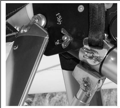
Allow the main tube to rise by loosening the strap until high enough to connect the universal junction to the wing. Insert the bolt with bolt head retaining unit. Tighten wing nut firmly and secure safety pin. The wing should only be attached using the central hole on the U-bracket as shown. Remove mast retaining strap.
