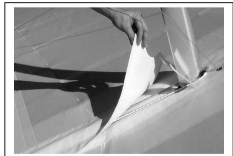
Figure 32 Section 4. Remove Sail Cowling
