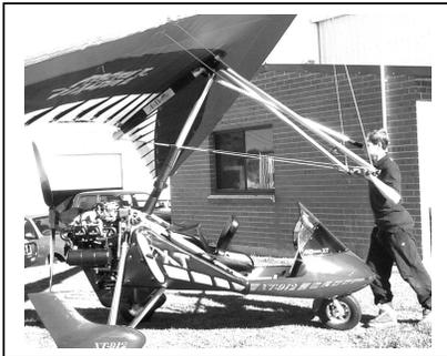
Go to the nose of the wing and with the mast brace tube in one hand and the control bar in the other lift the base bar. Rotate the wing until the rear of the keel rests on the mast. In strong winds maintain a firm grip on the wing.
