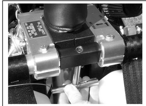
Figure 21 Section 4. Load Mast Lever
