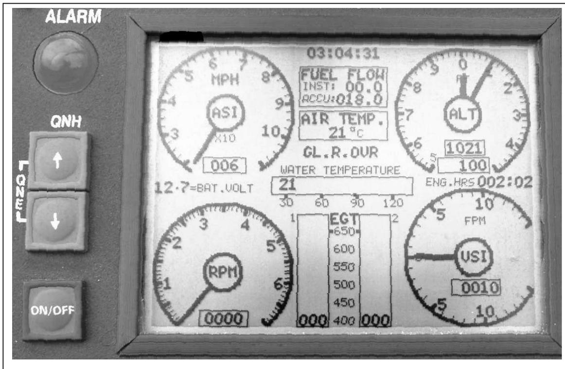
Figure 4 Section 7. GX2 Display
