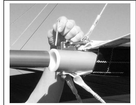
Figure 17 Section 4. Remove Keel Extension
