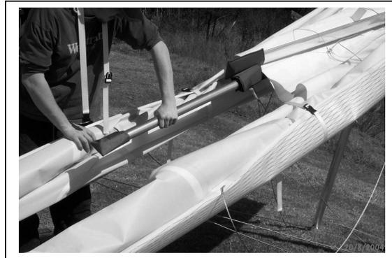
Figure 36 Section 4. Fold Leading Edges
