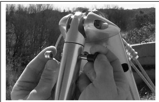
Depress pip pin button and remove pip pin from base bar. Fold down tubes together with base bar folded out. Reinsert the pip pin.
