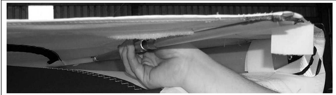
Figure 12 Section 4. Load Tip Strut
