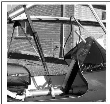
The mast has a gas assist strut to assist lifting the wing when the mast is raised. To hold the mast in position for wing attachment the mast retaining strap should be routed around the rear steering bracket and over the mast. The strap can be adjusted to pull the mast down to the correct height.
