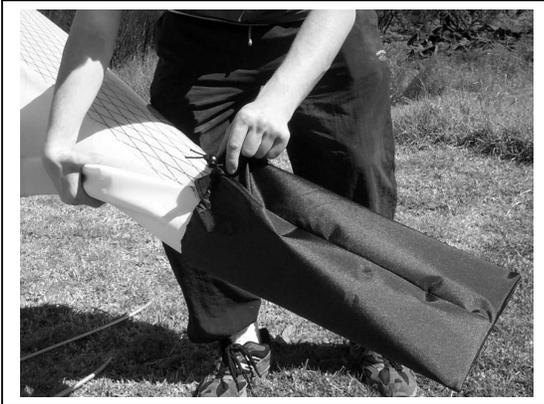
Roll sail at the tips inwards and parallel to the leading edge. Slide the tip bag over the end of the leading edge. The barrel lock unit can be used to tension the bag bungee.
