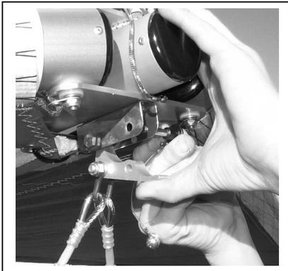
Remove the nose cone. Disconnect nose catch by removing the pip pin. The pip pin button should be depressed with the thumb while simultaneously pulling the pip pin out. Re-insert pip pin in nose channel.
