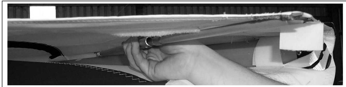
Figure 24 Section 4. Detension Tip Strut
