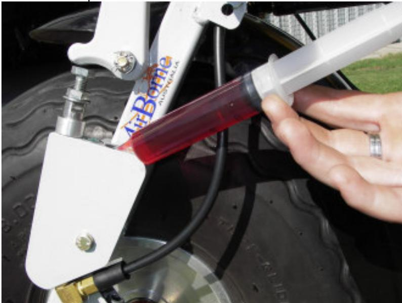
Figure 2 Brake fluid top up
