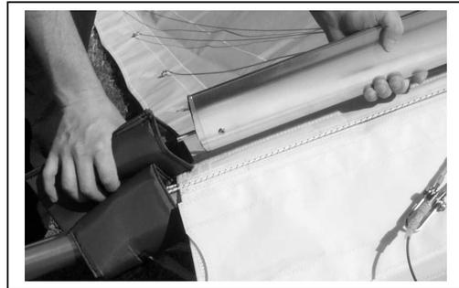
Remove the king post by lifting upward. Fit the quick clip king post base cover around the quick clip. Insert the king post in to pouch.
