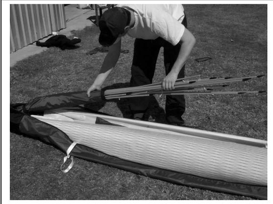
Stow the battens with the curve down at the rear of the glider bag. Reattach wing straps so that the control frame and battens are within the leading edge pockets. Zip up the wing bag.
