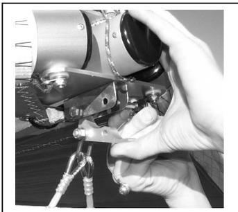
The nose catch should now be attached so that the pip pin is inserted through both the nose catch and channel. Ensure the pip pin cap is secure.
