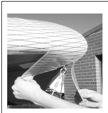
Attach the nose fairing by applying the top Velcro first then gently tension over the nose plates and attach the Velcro to the undersurface.
