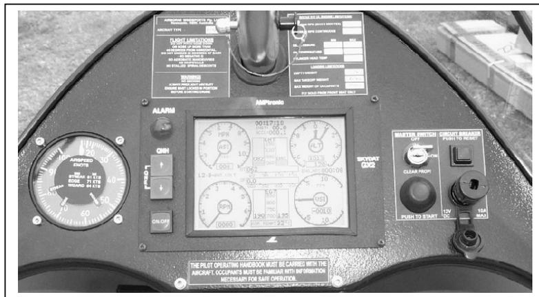
The instrument panel consists of an analogue airspeed indicator (knots) on the left side with the digital GX2 instrument mounted centrally in the dash. A power circuit breaker, power switch, 12V DC outlet and starter switch, can be found on the right side of the dash.
