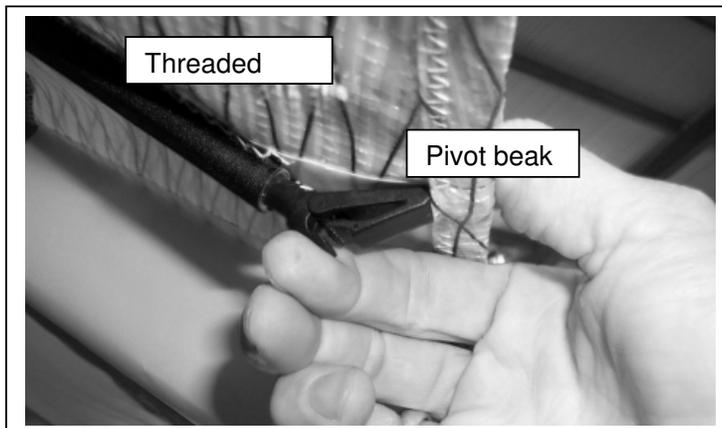
Remove outermost three tip battens. Unclip 'pivot beak' from 'threaded end'. Rotate *pivot beak* and remove from sail as shown. To adjust batten load tension, release *pivot beak* from sail and rotate batten clip. See maintenance manual for adjustment details.
